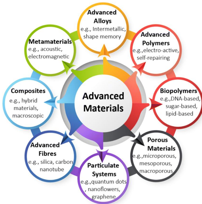
Fig.1: Broad classification of advanced materials by German Environment Agency (Ref. Source: Environ. Sci.: Adv., 2023, 2, 162)
